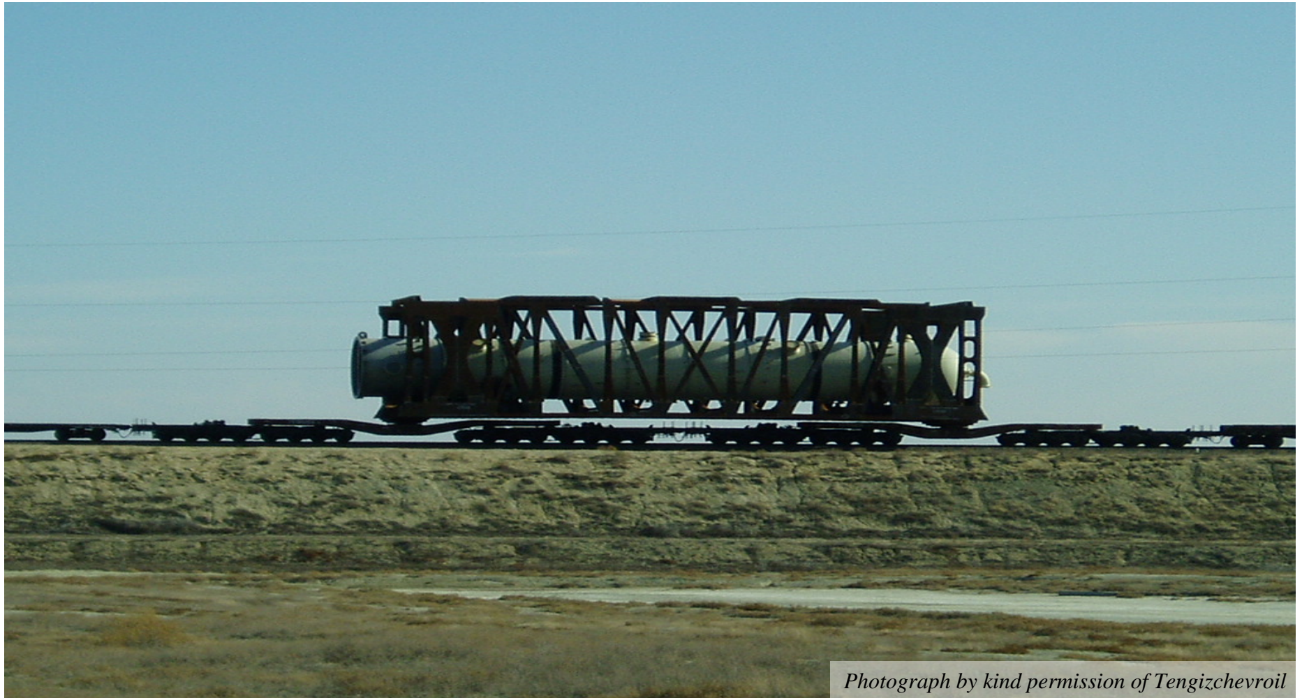
Photo 3: Large equipment on specially constructed transportation frame
